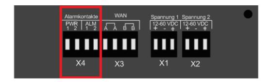
The Alarm contacts are used by connecting an electric circuit to the screw connector if an alarm is engaged the power (PWR) alarm relays is opened and the WAN (ALM) relays is closed.
