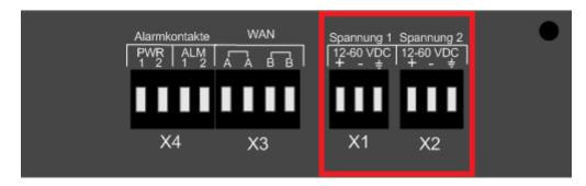
This unit has a redundant power supply. This means i.e. you can have 24VDC on screw connector PWR-1 and 48VDC on PWR-2. If one of the power sources fails, the other one will immediately take over.
