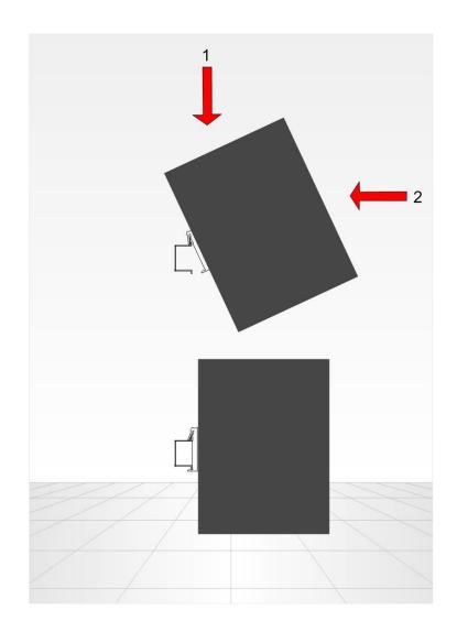
This unit should be mounted on 35 mm DIN-rail, which is horizontally mounted inside an apparatus cabinet, or similar. Snap on mounting, see figure. To cool this unit convection cooling is used. To avoid obstructing the airflow around the unit, use the following spacing rules. Minimum spacing 25mm (1.0 inch) above / below and 10mm (0.4 inches)
